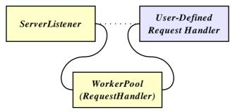
*WorkerPool* distributes the requests to workers that process them with a userdefined request handler using exactly the same process() interfaces of *RequestHandler* class as without the distribution.
