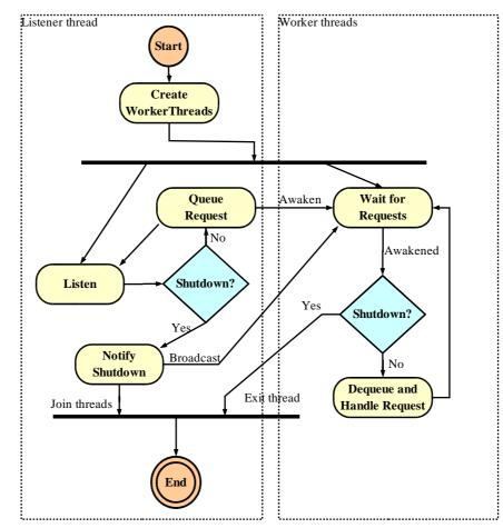
The requests are queued in the listener thread. The threads normally sleep in wait state, waiting for a signal. When the listener thread inserts a request in the queue, it awakens one of the sleeping threads to process the request. Also, when the main
