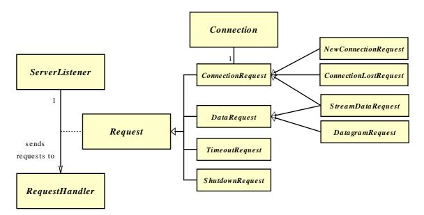
The *ConnectionRequest* class is associated with an established TCP client connection object, to provide its inheritors access to that object. The abstract *DataRequest* class contains a data buffer containing request data read from the socket by *ServerListener*.
