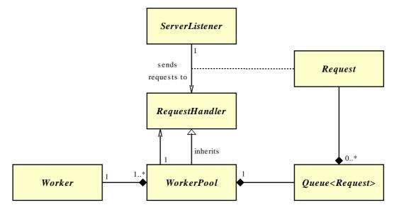
The *RequestHandler* referred by the *ServerListener* is a *WorkerPool*, which in turn refers to a user-defined sub-class of *RequestHandler*. Each of the *Worker* objects have an execution method that executes in its own thread, reading requests from the queue and passing the to the user-defined request handler.
