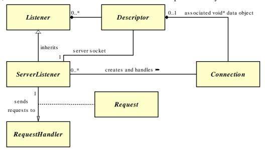
The descriptors handled by the *Listener* can actually be any file descriptors such as files, pipes, or sockets. The *Listener* class doesn't know anything about sockets or socket types (server or client) or *Connection* objects. These are semantics attached to the descriptors and their associated data by the *ServerListener* class.
