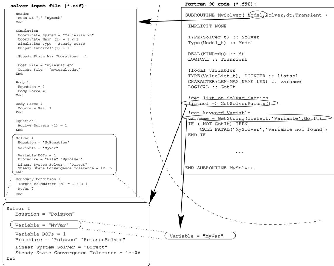
Figure 19.1: Scheme of the access of structures in the solver input file from a Fortran 90 user subroutine. The example shows, how a string is read in from the Solver section.
