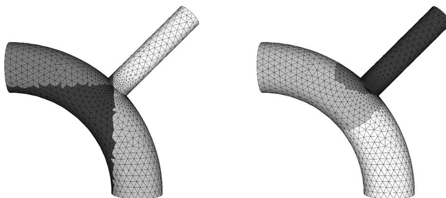
Figure 17.2: Distribution of four partitions using the options `-partition 2 2 1` (left) and `-metisway 4` (right). It comes clear that the partitioning to the left contains more partition-partition boundaries and consequently will perform worse in a parallel run
