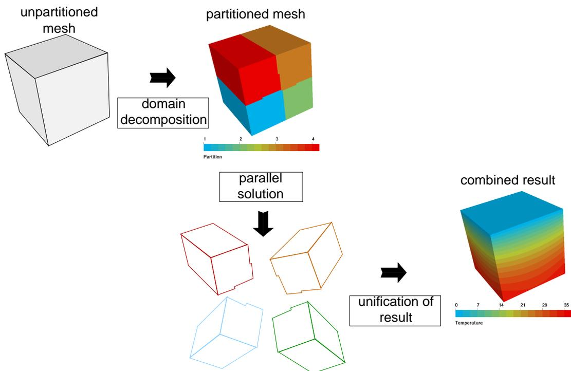
Figure 17.1: The principle steps to be taken for a parallel run of Elmer
