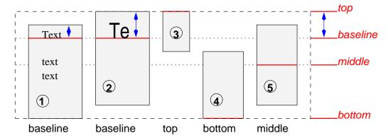
Diagram showing the effect of various values of 'vertical-align' on table cells.
